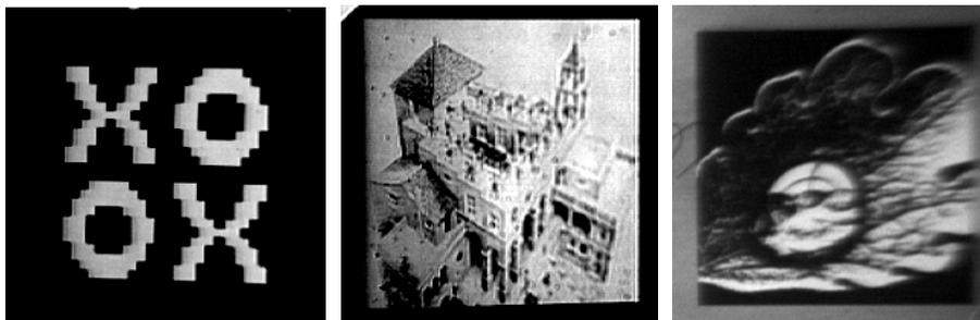
**Figure 3. MWIR images from LCOS displays (blackbody source).**
