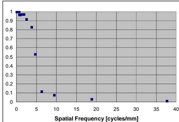
**Figure 4.** Measured MTF of the UCF nematic display.
