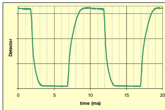
**Figure 5.** Switching response of the MWIR FLC cell.
