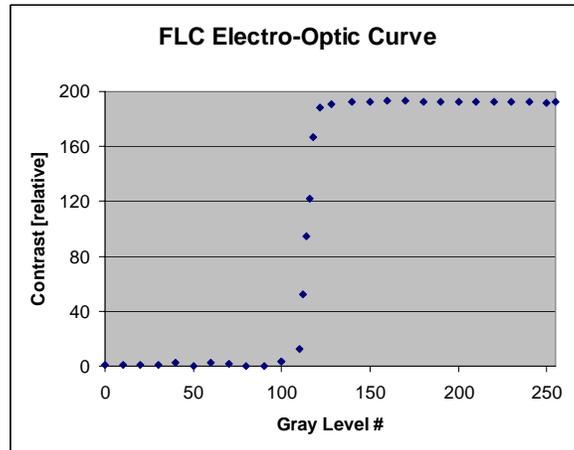
**Figure 8. Grayscale response of the FLC display.**
