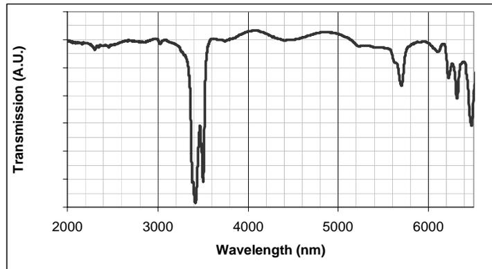
**Figure 6. Transmission spectrum of the FLC cell.**
