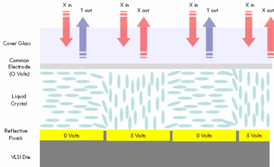
**Figure 1.** Side view of a LCOS display.
